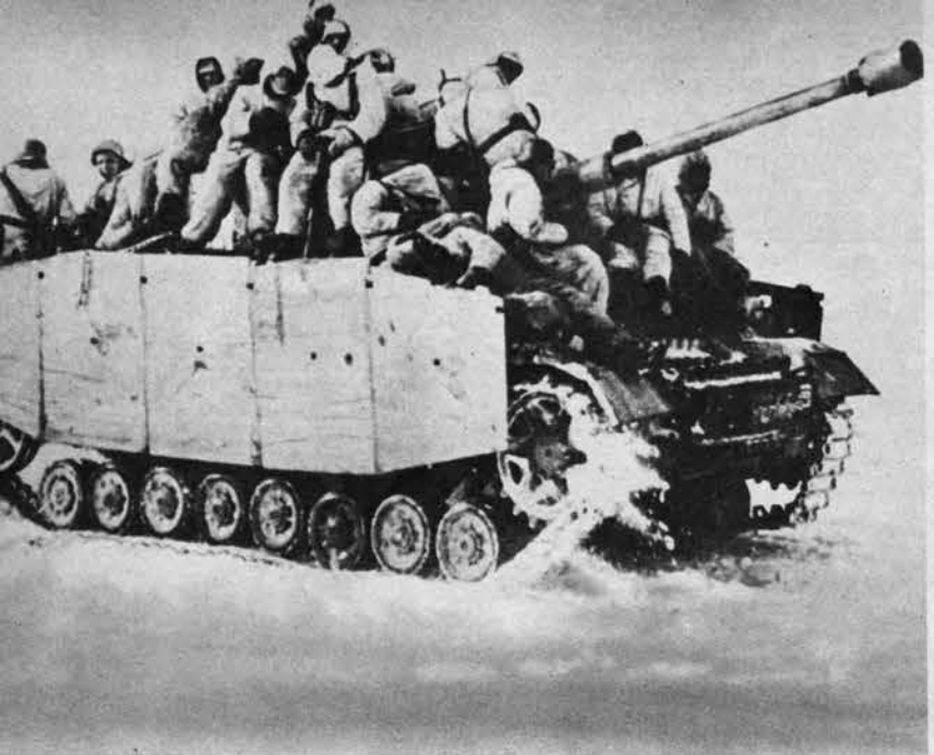
Nazi soldiers cluster on top of a PzKw IV tank. Armored side skirting, bracketed to Mark IV's chassis, alters the appearance of the undercarriage, leaves only the sprocket and eight small wheels exposed.
